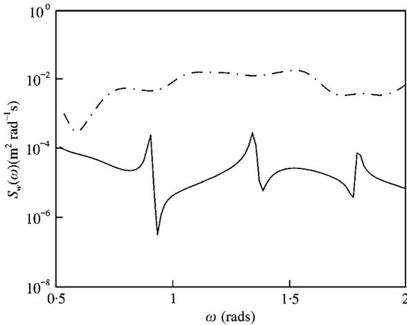
Figure 13.  $S_w(\omega)$  at  $s = L/2$ : —, with friction damping; - · - · -, without friction damping.
