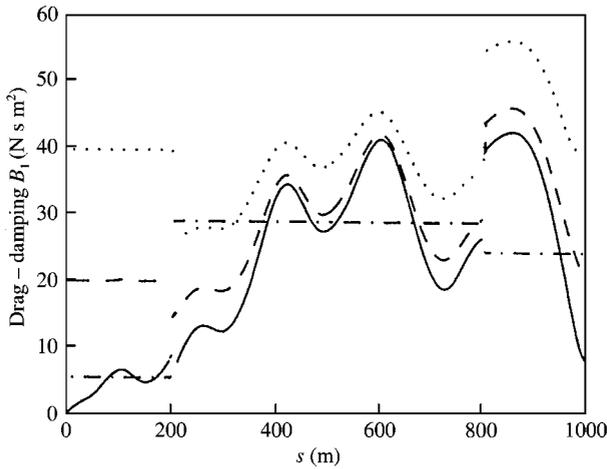
Figure 10. Drag on composite cable —, actual; - · - · -, segmentwise constant; ---, current effect ( $V_1 = 0.25$  m/s) and · · ·, current effect ( $V_1 = 0.5$  m/s).
