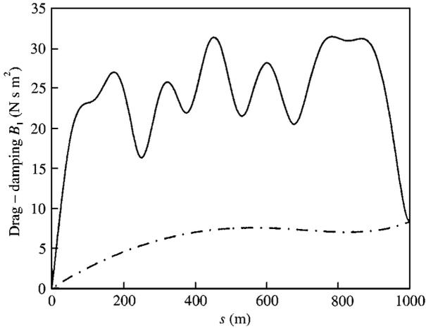
Figure 3. Effect of dynamic and quasistatic analysis: —, *dynamic*; - · - · -, *quasistatic*.
