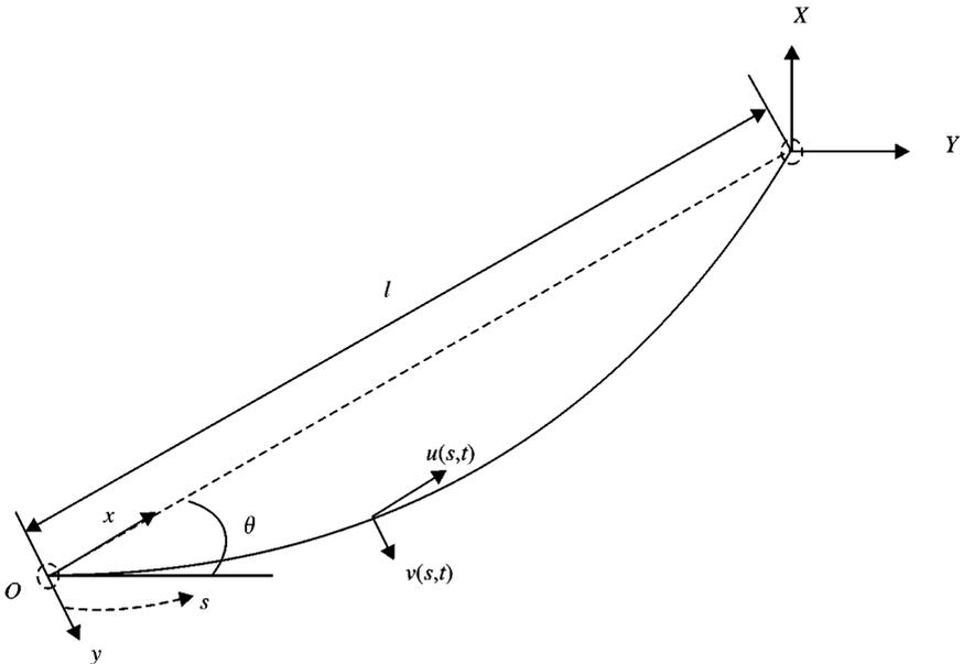
Figure 1. Schematic diagram of a mooring cable.
