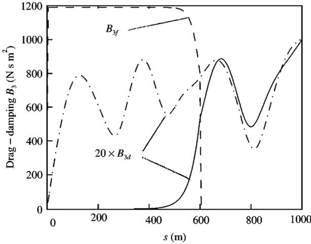
Figure 12. Drag fiction damping: —, drag damping; ---, friction damping; - · - · -, drag damping without friction damping.
